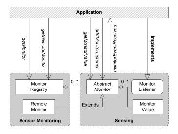
Fig. 2. The internal class diagrams of the sensor monitoring and sensing components of CONSUL
