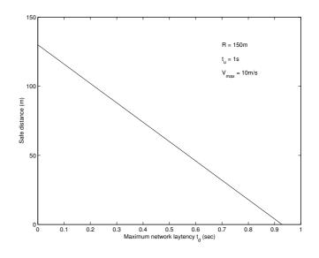
Figure 10: Safe distance vs. network delay
