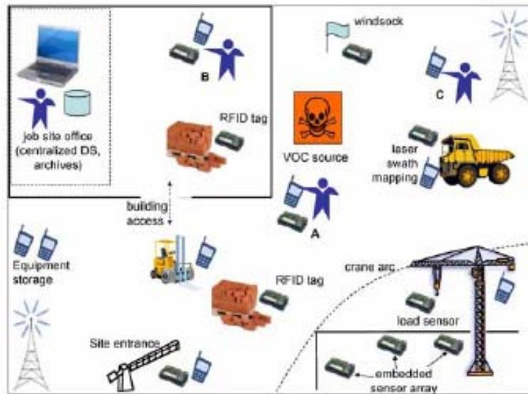
Figure 1: A representation of applications on the Intelligent Job Site
