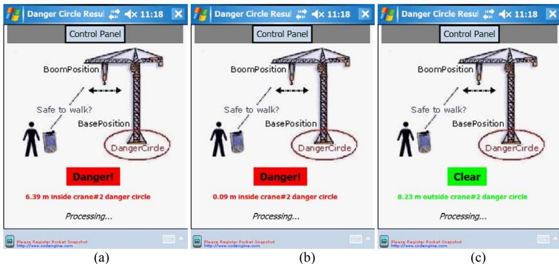
Figure 5: Example deployment of crane movement warning
