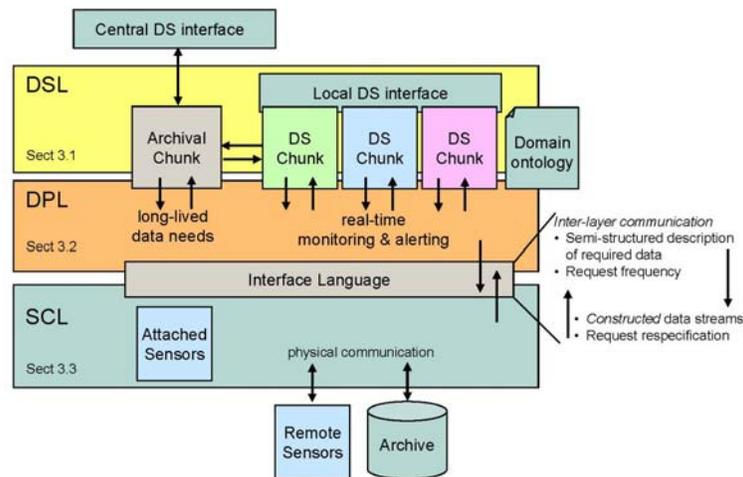
Figure 2: Three-layer architecture for decision support in ad hoc sensor networks
