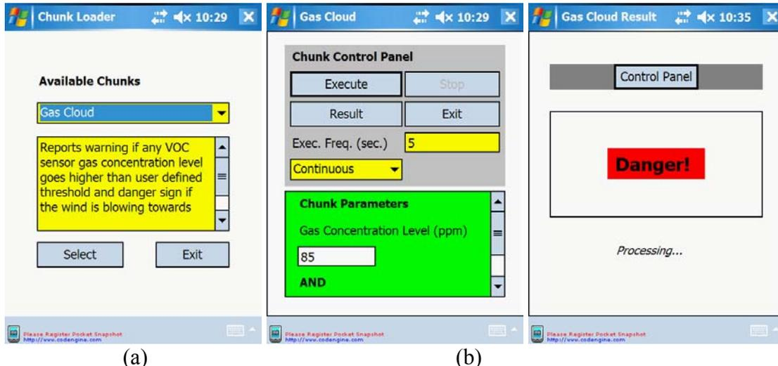
Figure 3: User interface of VOC detection application
