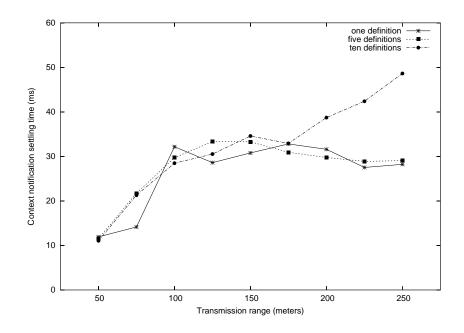
Fig. 10. Maximum time for last context recipient to receive notification for varying network loads
