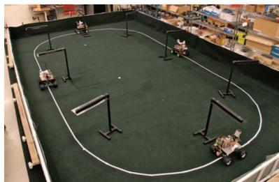
Fig. 6. The multi-robot patrol testbed.
