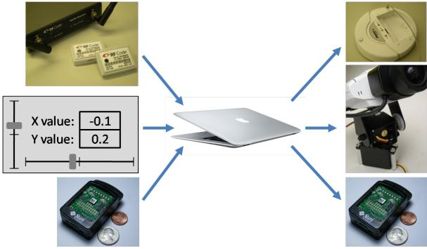
**Figure 2:** Flow of data among devices in demonstration. On the left are *sensors*, on the right are *actuators*, and in the center is the SEAP server.
