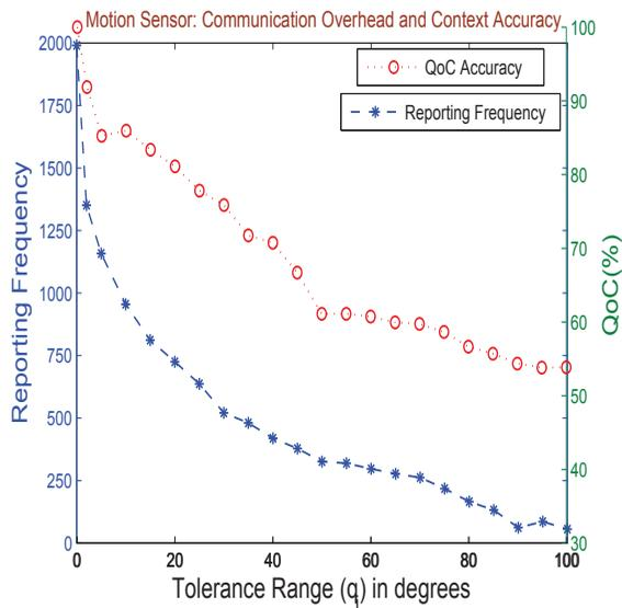
Fig. 5. Communication Overhead and QoC accuracy vs. Tolerance Range using Motion Sensor
