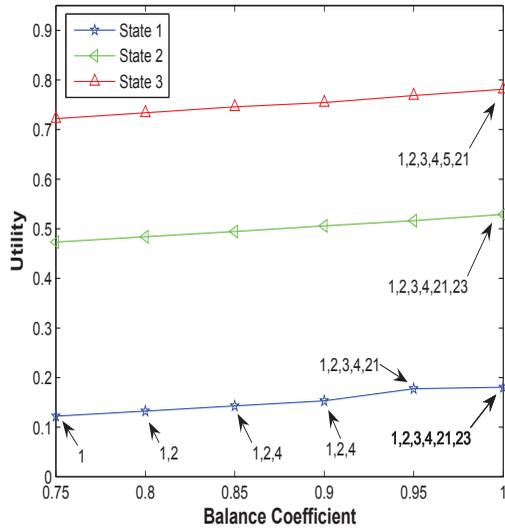
Fig. 10. Utility values (Best Sensor Subset) for different values of balance coefficient  $\alpha$
