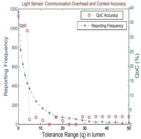
Fig. 6. Communication Overhead and QoC accuracy vs. Tolerance Range using Light Sensor
